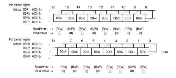
Note: No register bit is included in bits 7 and 6 of port 7 or bits 7 to 3 of port 8. Port 6 has no DDR.
