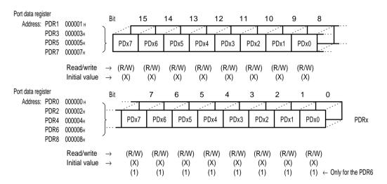
Note: No register bit is included in bits 7 and 6 of port 7 or bits 7 to 3 of port 8.
